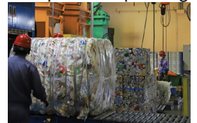
Plastic containers and packaging that become a bale (mass) of around 260 kg.
