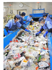
Hand sorting conveyor for plastic containers and packaging (left) manually sorts out foreign materials.
